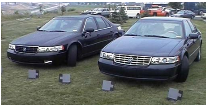
Figure 1. Fixed and swiveling headlamp test vehicles with targets.
